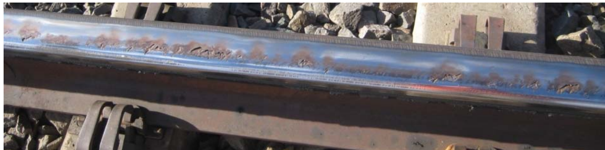
Dye Penetrant Photograph of Rail in Revenue Service
